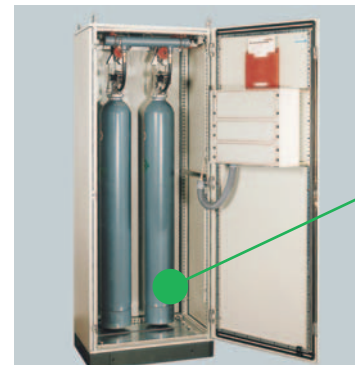
Nitrogen gas cylinders of the Argotec compact extinguishing system are pressurised to 300 bar, so that the weight and space requirements are minimised
